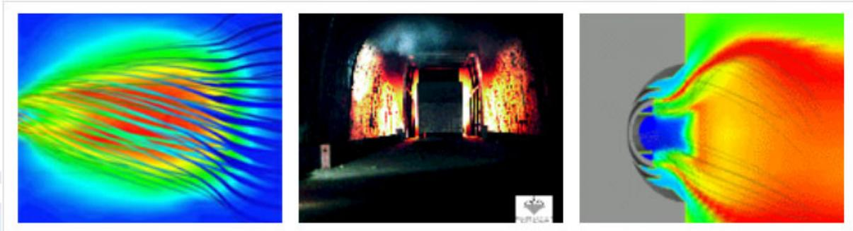
CFX simulation of the air flow and gas temperature in a swirling turbulent diffusion flame
