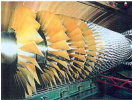
Siemens 15 stage axial compressor
